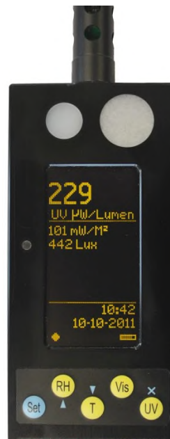
Elsec 765C data logger for accurate monitoring of environmental conditions
