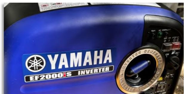
Generator for dehumidifiers in case of prolonged power outage
